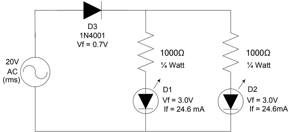
Figure 6 – LEDs in a parallel circuit
