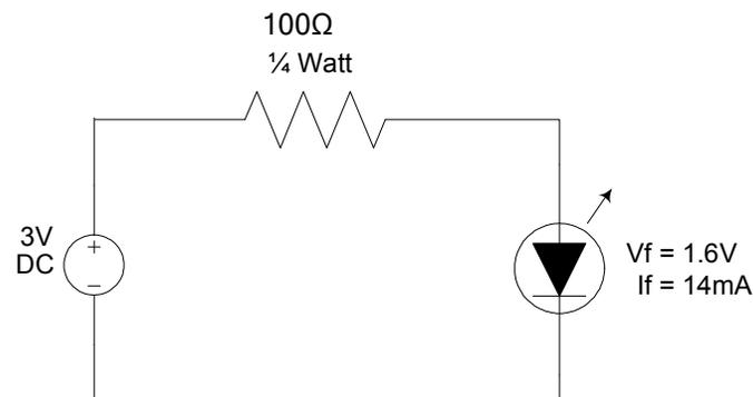
Figure 8 – Circuit using 3 volt DC supply and LED with 1.6Vf
