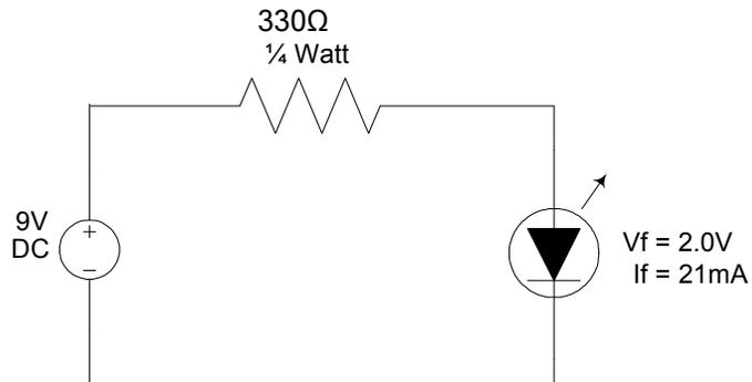
Figure 7 – Circuit using 9 volt DC supply and LED with 2.0Vf
