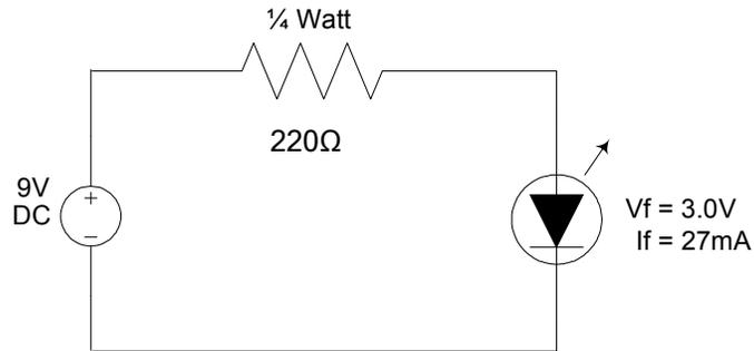
**Figure 4 – Example circuit**
