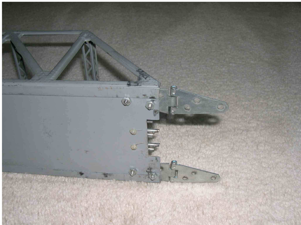
Photo #8 -- Bridge #2 – Lionel #317 – Bottom showing cutout
