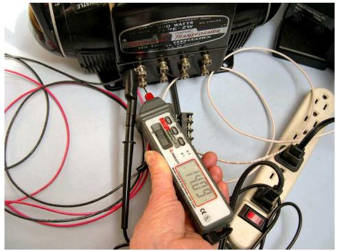
Figure 2 – Voltage output of a ZW Transformer with throttle set at 14 volts
